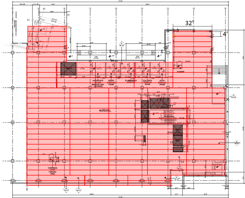
Figure 6: Hollow Core Plank Breakdown of First Floor West End (plans provided by HDR, Inc.)
