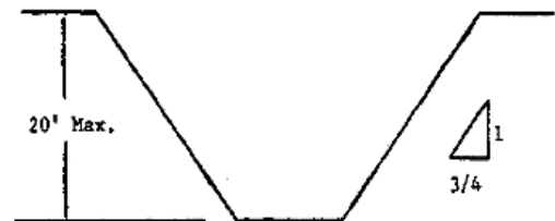
Figure 45: Section View of Excavation of Soil Class A (image provided by OSHA)
